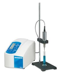
**Stand and Converter Holder:** The support stand with stainless steel rod accommodates Branson's 20 kHz converter. The converter holder supports the ultrasonic stack (converter and horn) and is adjusted easily to properly position the horn in the sample.
