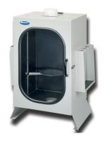
Acoustic Enclosure: Operating a Sonifier SFX Series in the Soundproof Enclosure can minimize mechanical noise produced by ultrasonic processing. The sturdy cabinet is lined with waterproof, sound-absorbing material, which is impervious to most solutions or laboratory reagents and can be cleaned easily. A fully-transparent door enables viewing of the process while limiting the noise to an acceptable level.
