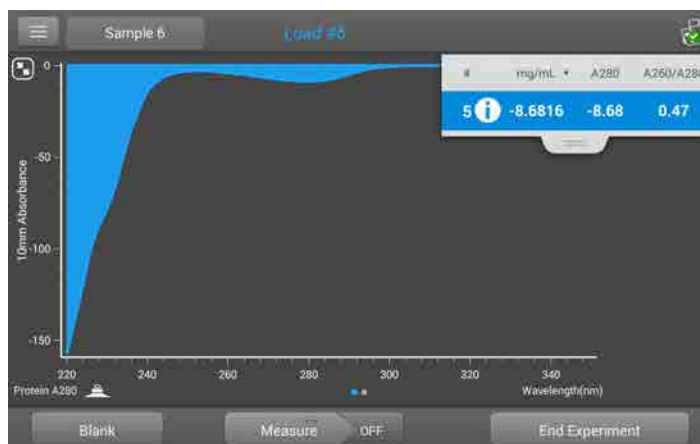
Protein sample solution used to blank instrument results in “mirror image” spectrum
