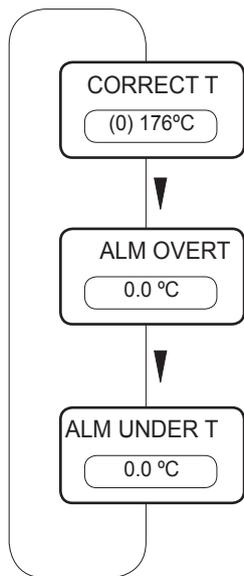
Fig 7.2. Temperature alarms
