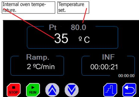
Fig 7.3.1. Run screen operating at one temperature.
