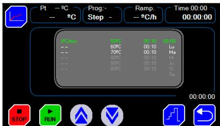
Fig 7.3. Run screen operating with temperature profile.
