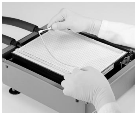
Fig 32. Positioning equilibrated IPG strips on Multiphor II.
