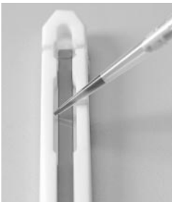
Fig 19. Applying sample after gel rehydration.
