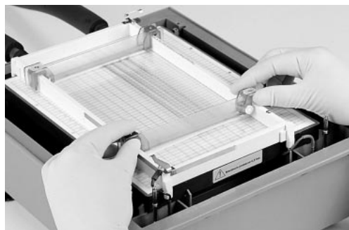
Fig 13. Alignment of electrodes over IPG strips.
