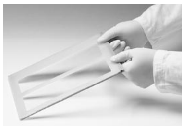
Fig 26. Closing the Precast Gel Cassette.
