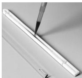
Fig 17. Applying rehydration solution into the strip holder.
